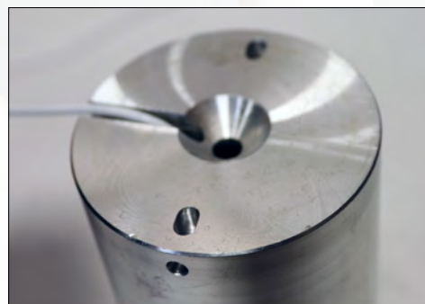
STS-102 A 035 sensor in an insert.
